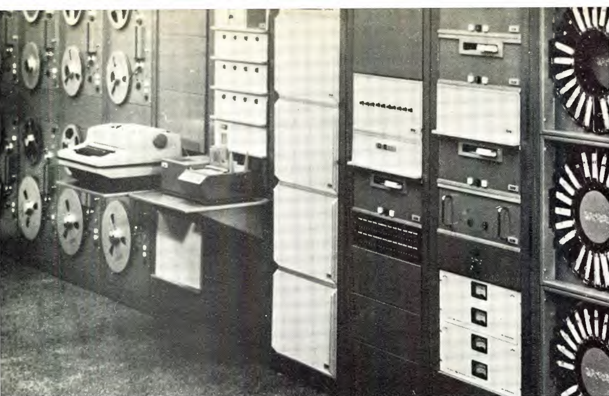
Fig. 3 The IGM 600 system uses a card reader to input program information. The typewriter produces a log by typing out the information on the card as it is read by the system. The typewriter also is used to make real-time changes or corrections to the log.
